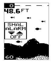
Press the down arrow key to silence the alarm. This will turn the alarm sound off until the shallow alarm is triggered again.
